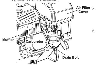
b. Remove the drain bolt from the bottom of the carburetor bowl and allow the fuel to drain.
